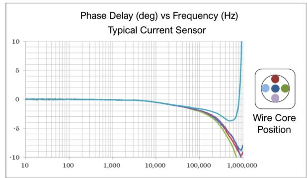
Figure 7: Typical sensor's phase delay and wire position
