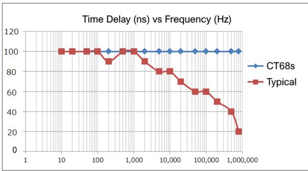
Figure 4: Typical sensors compared to HIOKI CT68 series
