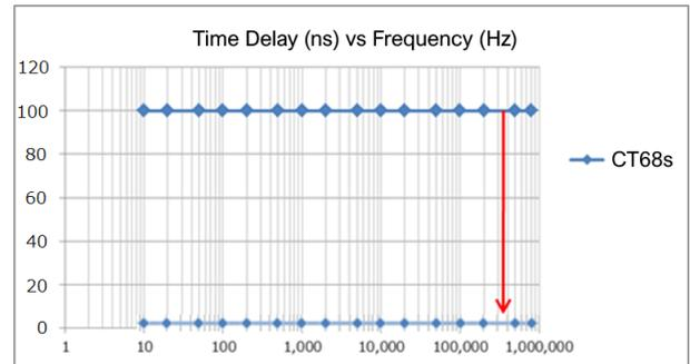
Figure 2: Time delay of HIOKI CT68 sensors
