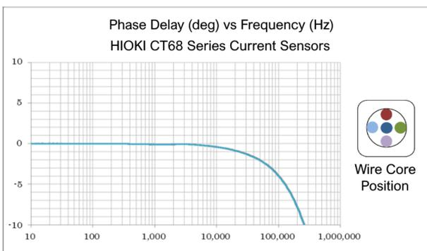
Figure 6: HIOKI CT68's phase delay and wire core position
